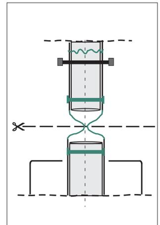
Figure 3: Sealing of the protection tube
