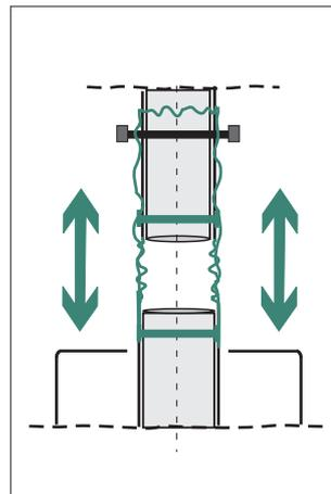
Figure 2: Filter cartridge with extraction pipe and extendable flexible protection tube
