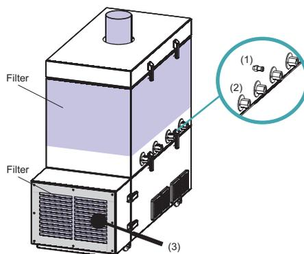
Figure 4: Integrated product features for qualification of the device in the production area (1: overpressure measuring on tightness; 2: qualification measurement behind the main filter)
